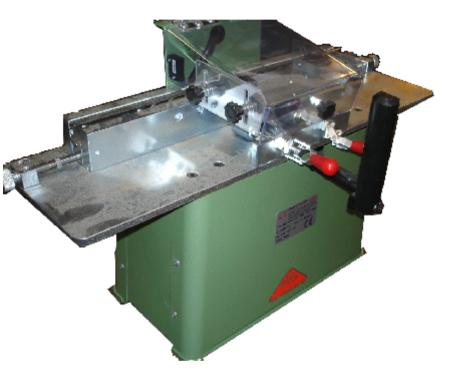
The perfect machine for producing the half-lap joint as found in Georgian window bars. It is used for both "plant-on cassettes" and rebated bars.
